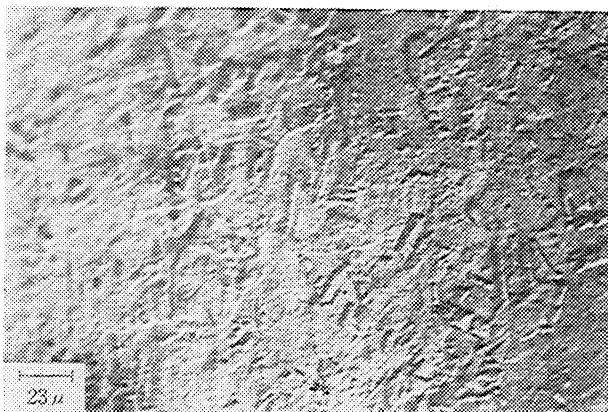
Photo. 1—3. Surface of nickel deposit obtained from Ni(CF 3 COO) 2 (100 g)/HCONH 2 (1 l) bath at 1.0 A/dm 2 at 60 °C.
